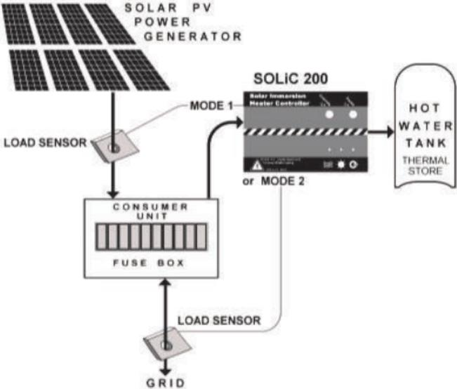
Fig 1 - Installation differences between mode 1 and 2
